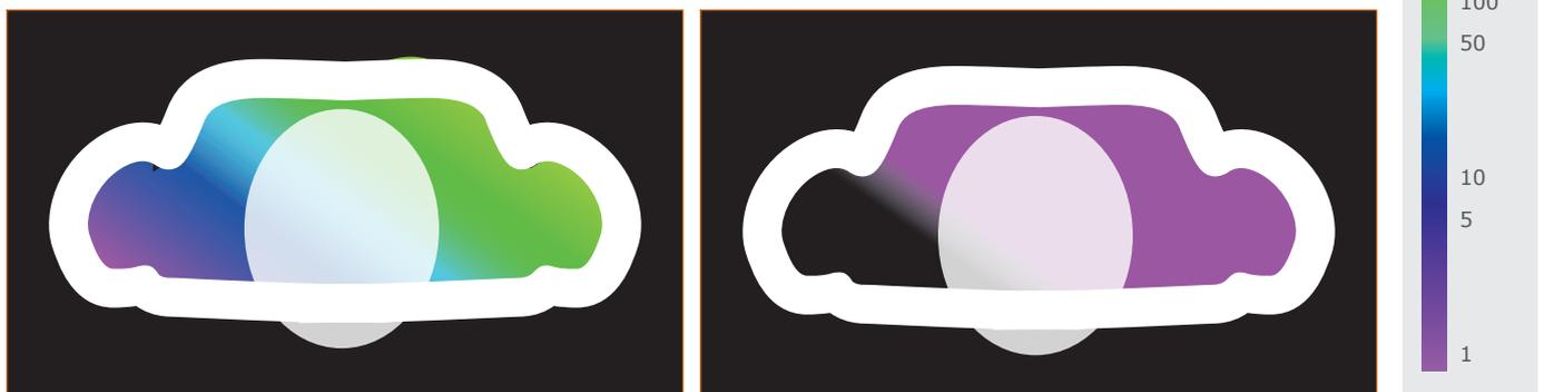
Fig.3.a Situation for the examiner with the new protective shield *without* a curtain: The light blue area indicates a high exposure dose in the upper body area as a result of the radiation that has traveled underneath the radiation protective shield.
