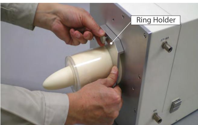
And then, put the ring holder around the base of the phantom and fix it to the machine unit with a screw.
